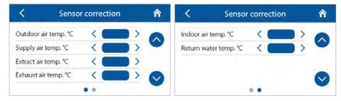
The sensor readings are corrected by entering values with horizontal arrow keys in the range from -50.0  $^{\circ}$ C to +50.0  $^{\circ}$ C.
