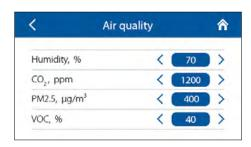
Set threshold values for the humidity, CO<sub>2</sub>, PM2.5, and VOC sensors. The unit will automatically maintain the user values by smoothly increasing or decreasing the fan speed.
